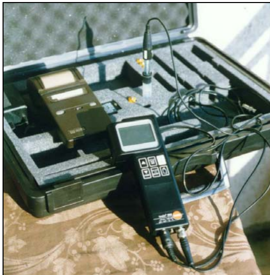
Measurement equipment for in situ investigations of water samples
