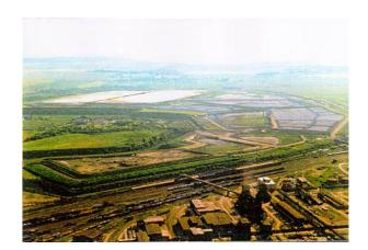
The industrial waste disposal site is situated in the mining and industrial area of Halle and Merseburg. It covers about 300 ha and is the largest waste disposal facility in Germany. The site went in operation already in 1937 and served for the evacuation of all industrial wastes generated in the area, such as industrial water treatment sludges, coal power plant ashes and carbon hydrates.
