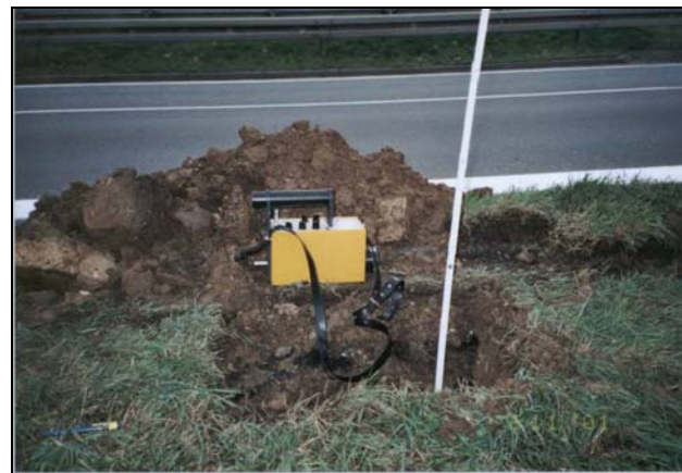
digging for sampling and dose rate measurements
