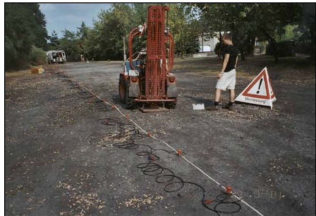
Seismic measurements for localisation of cavities
